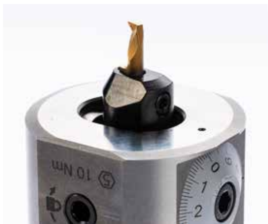
normal (rechte Schneidplatte) normal (right hand insert)
